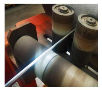
Bare wire annealing. Annealing is a process at high temperature which aim to soften the copper and make it more malleable.
