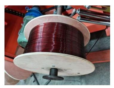
Coils winding. Once is ended the wire enameling, the wire is assemblied in particular spools to be later on weighed and sold.
