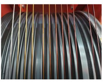
LP Industry can produces custom round, square and rectangular wire in a well equipped, fully permitted manufacturing facility. Products offered include film insulated wire conforming to NEMA MW 1000 and IEC60317 in temperature classes 105 °C to 240 °C, from single through double film builds. Low minimums, quick deliveries and top quality are our standards.
