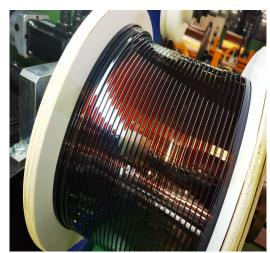
**Good electrical conductivity**: Enameled flat copper wire has excellent electrical conductivity due to its high purity copper core, which makes it an ideal choice for electrical applications.
